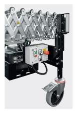
The flexible roller conveyor is operated via a switch console at the start of the conveyor, located below the scissor elements.
