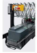
The classic control cabinet is no longer required. The frequency inverter is integrated in a drawer and can be pulled out from the side. Emergency stop switches are located at the start and end of the conveyor and at every 12,000 mm.
